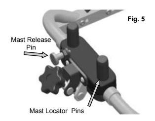
5. Place mast assembly over locator pins on base assembly (fig 5). Rotate locking pin until it engages into mast assembly. Make sure that the mast pin is fully engaged and holding the mast firmly to the base (fig 6). If the mast lifts up from the base, twist the retaining pin again making sure that the pin fully engages into the mast assembly.
